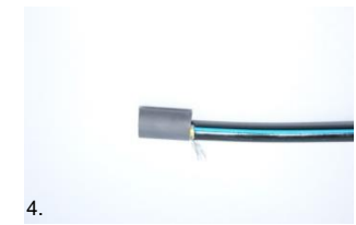
4. Pull the 30 mm long heat shrink tubing over the end. Shrink it down
