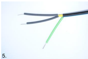
5. Pull the two slim heat shrink tubings over the copper conductors and the yellow/green one over the twined earth wire. Heat and shrink down
