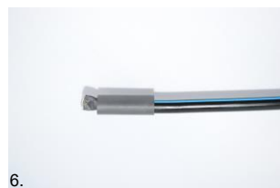
6. Wrap the Mastic tape 19x30 mm around the cable until it overlaps the outer sheath and the inner shrink tube
