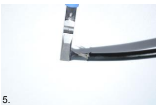
5. Pinch the end of the heat shrink tubing with small, flat plier.
