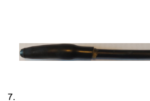
7. Fold the pinched end of the tubing inwards and pull the larger heat shrink tubing over the end until it overlaps the outer sheath with min. 20mm. Shrink it down until glue is pressed out of the tubing
